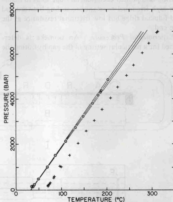
FIG. 4. Data points obtained with "J" dilatometer for determination of two isomekes between quartz  $\perp c$  and quartz  $\parallel c$ . The intermediate straight line associated with the set of experimental points denoted by circles was determined using Equation (7-II) and data at 25°C and atmospheric pressure from McSkimin *et al.* (1965). Straddling lines indicate standard deviation of slope based on estimated standard deviations of properties used in Equation (7-II).
