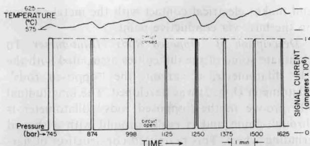
FIG. 3. Part of 2-pen strip chart record for determination of an isomeke between quartz (48° from  $c$ ) and almandine using the "J" dilatometer. Corrected for offset of pens.
