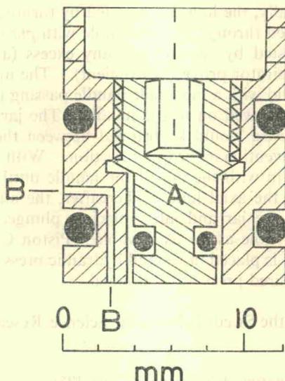
FIG. 2. An O-ring plug for the optical cell
